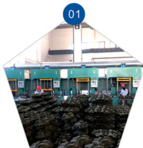
覆膜砂铸造制壳
